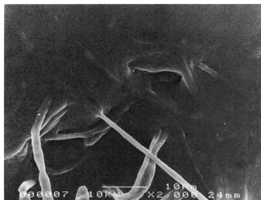
Figure 7 Electron micrograph showing filamentous fungi developed at the surface and through the bulk of racemic PLA plates buried 8 weeks in soil and then incubated 8 weeks in a Petri dish containing mineral agar medium.
