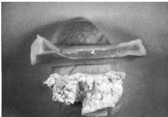
Figure 3 Cross-sections of racemic PLA plates at 32 weeks of aging in control (above) and in microbial liquid media.
